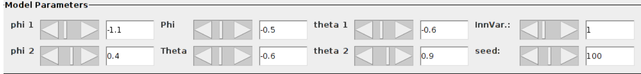
Figure 9: Once changes to one of the values has been made, the data is re-plotted keeping all other parameters, including the random number generator seed, fixed. This way, one is able to see how the dynamics of the underlying SARIMA model fluctuate according to small changes in the parameters.
